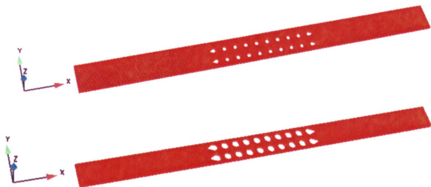
Figure 9.8. The finite element meshes of the HF (upper) and Bosch (lower) iDEP channels.
